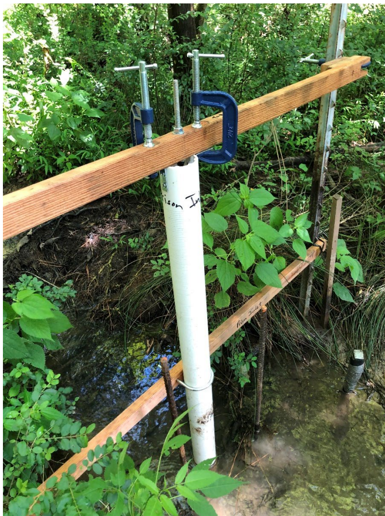
Figure 27. Apparatus for housing HOBO water level datalogger in small streams; metal stakes and cross braces connected to a standing PVC pipe with the HOBO unit suspended inside.
