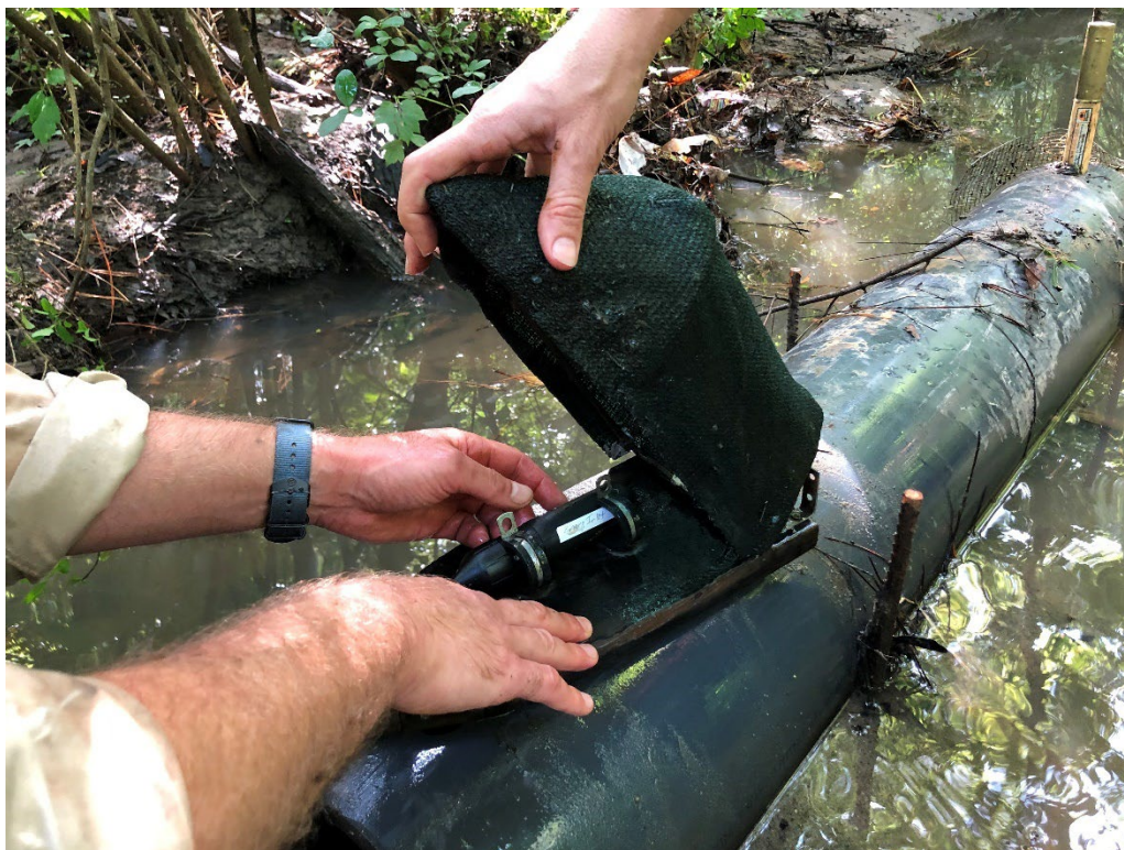
Figure 26. Apparatus for housing HOBO water level datalogger in flowing streams to prevent HOBO units from getting washed away; protective box was placed inside large pipe, which was staked in and had a screen at the upstream end to keep out debris.
