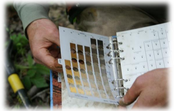
Wetland scientists use a Munsell Color Chart to determine soil types in wetlands.
